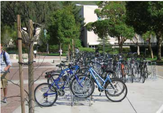
Higher-Density Racks such as the Peak Rack — Campus Rack can provide order and density
