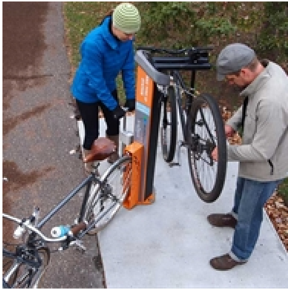
Example of a similar station with the seat post hanging device, tools, a pump, and a wheel chock.
