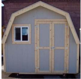
Pictured is a model of the storage sheds constructed by Ag Education students during the semester. It is a 10'x12'x8' gambrel-roof storage shed. The cost of these sheds are \$1000. If ordered for the MSU Child Development Center, the shed would be ready in January for installation in 2015.
